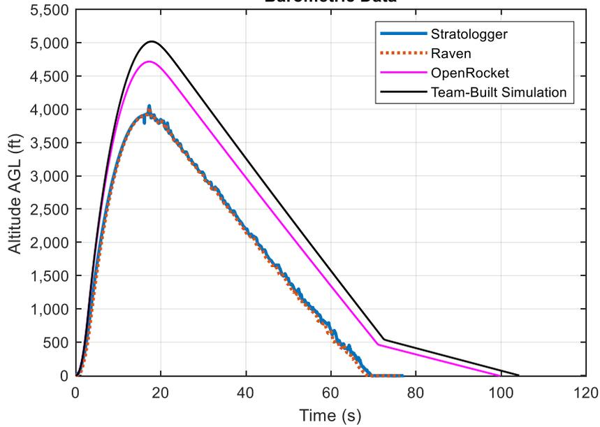
**Figure 1: Flight Profile - Full Scale Flight #1**
